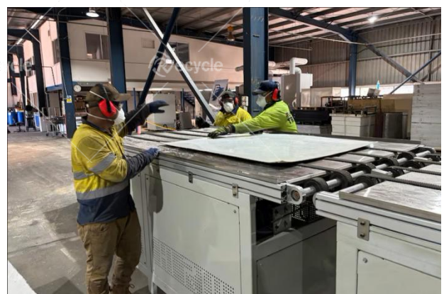
Solar Panel Recycling Line in Australia
